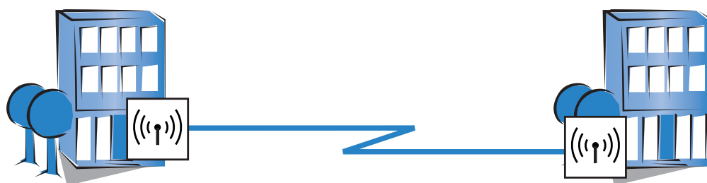
Figure 2: A wireless link between two access points
